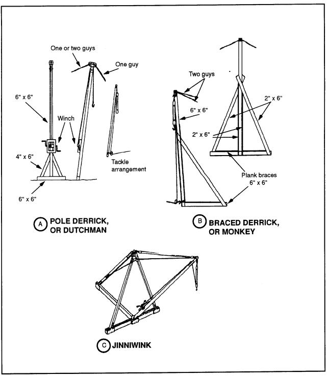
Figure 5-11. Light hoisting equipment
