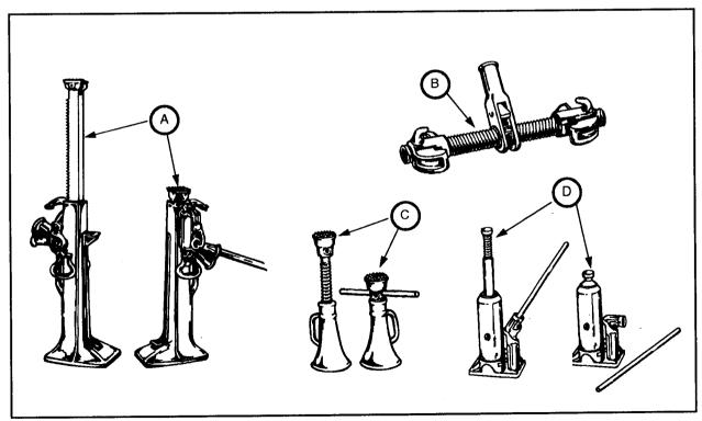
Figure 5-16. Mechanical and hydraulic jacks
