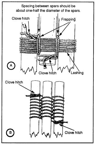
Figure 5-4. Lashing for a tripod
