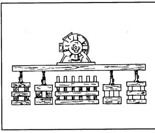
Figure 5-15. Jacking loads by stages
