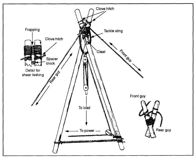
Figure 5-6. Lashing for shears
