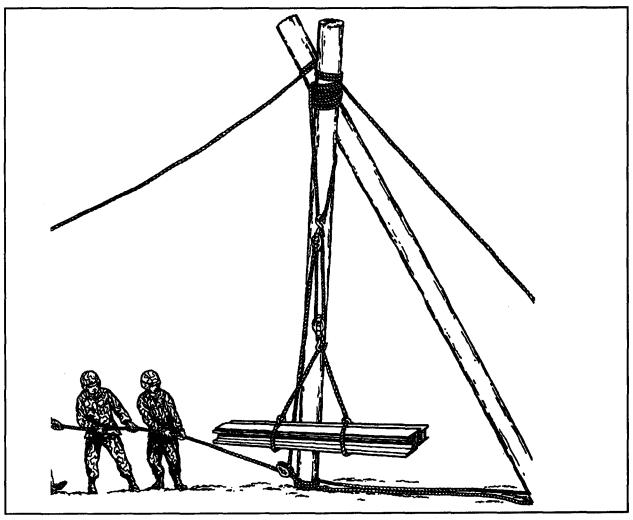
Figure 5-8. Hoisting with shears
