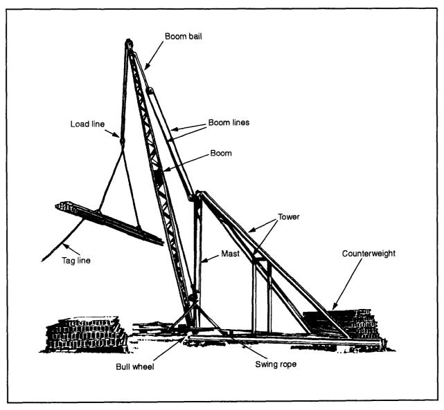
Figure 5-10. Four-ton stiff-leg derrick
