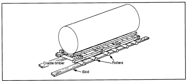
Figure 5-13. Using skids and rollers
