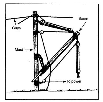
Figure 5-9. Rigging a boom on a gin pole
