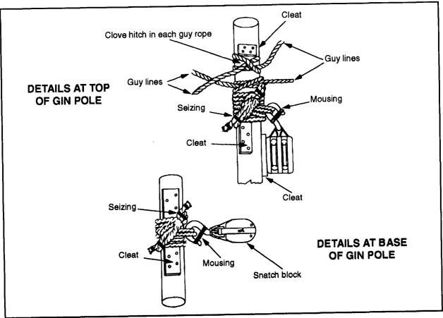
Figure 5-1. Lashing for a gin pole
