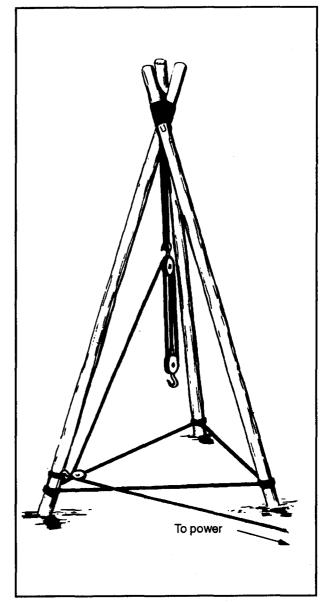
Figure 5-5. Assembled tripod
