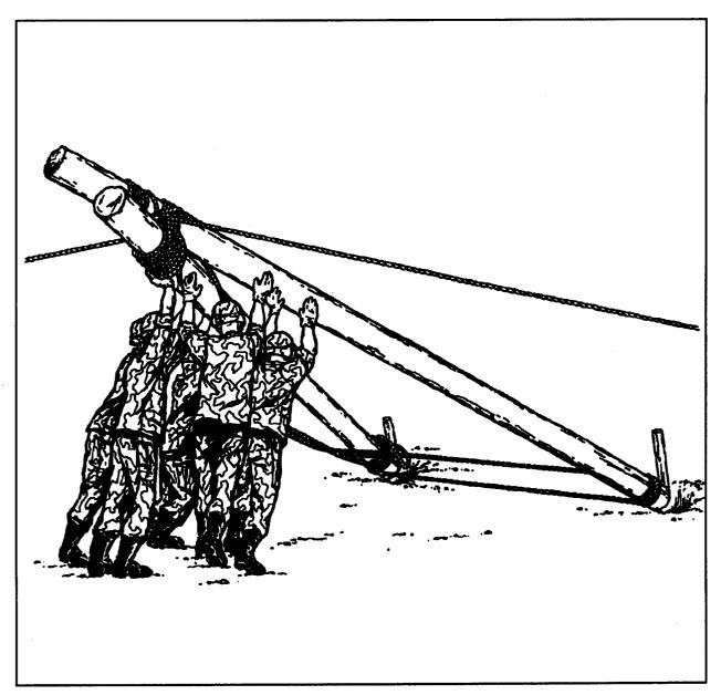
Figure 5-7. Erecting shears
