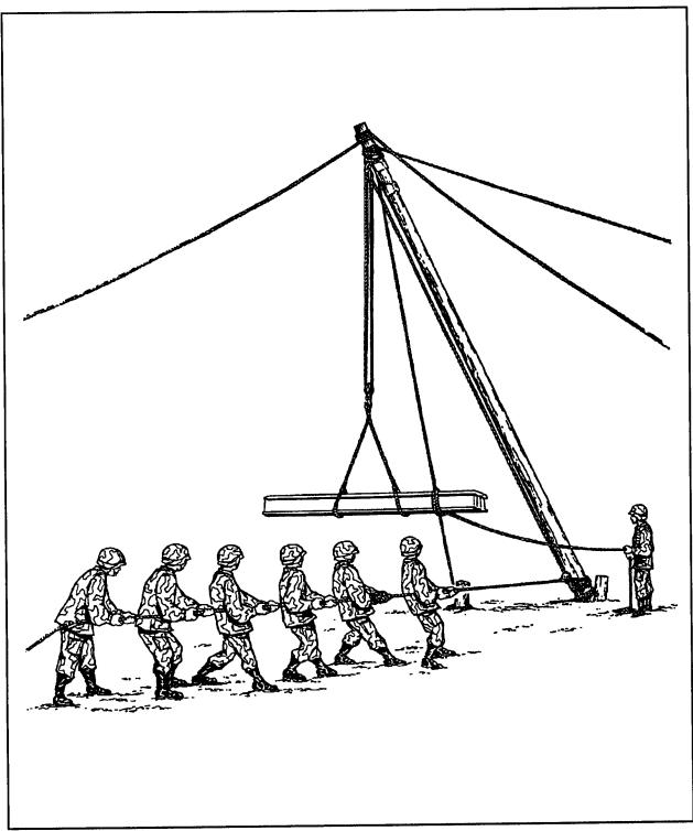
Figure 5-3. Hoisting with a gin pole
