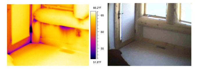
Figure 13 & 14. – Cooling patterns beneath log under window, at wood-to-wood joinery locations and along doorjamb. Cooling patterns illustrate air infiltration during blower door test. Note there is greater air infiltration under log than at electrical outlet in wall based on temperature differential.
