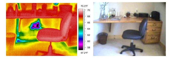
Figure 17 & 18. - Air infiltration at electrical outlet evidenced by significant cooling of outlet and surrounding materials during the blower door depressurization. Note that this indicates not only that a source for cold air in the logs behind this wall exists, but that the vapor retarder (if present) behind the drywall was not sealed at penetrations such as this outlet.
