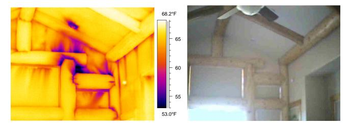
Figure 7 & 8. – Extensive air infiltration during depressurization at numerous wood-to-wood joinery locations where logs are exposed on interior of wall. Reference scale for temperature differential of 15.2°F between 68.2°F and 53.0°F.
