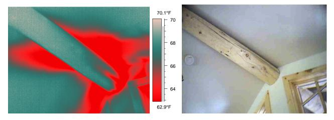
Figure 21 & 22. – Large cooling area clearly illustrates extent of air infiltration at top of beam where access is difficult and closure/sealing may have been altogether left out.
