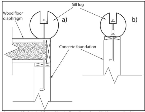
The test configuration included a Figure 2: Typical foundation details for log buildings; (a) sill log on floor diaphragm, (b) sill log on concrete foundation vertical load to mimic dead and live wall (from Scott et al. 2005a)
