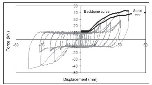
*Figure 3: Hysteresis diagram from a fully-reversed quasi-static test of a sill log on a floor diaphragm (from Scott et al. 2005a)*
