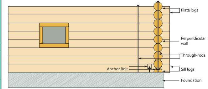
Figure 1: Log wall including a window opening and an inter-wall connection on a rigid foundation (from Scott et al. 2005a)
