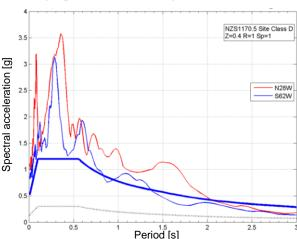
Figure 1: 5% damped elastic acceleration response spectra at the Te Mara Farm Waiau station (WTMC), horizontal PGA = 112% g, vertical PGA = 322% g. Solid line ULS, dotted line 0.25 ULS for soil class D [1]
