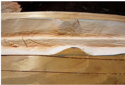
Figure 7.b: Tabs in a long groove that has been cut and sanded. (This is not the same log as Figure 7.a.) These tabs are about 1 inch (25mm) long.
