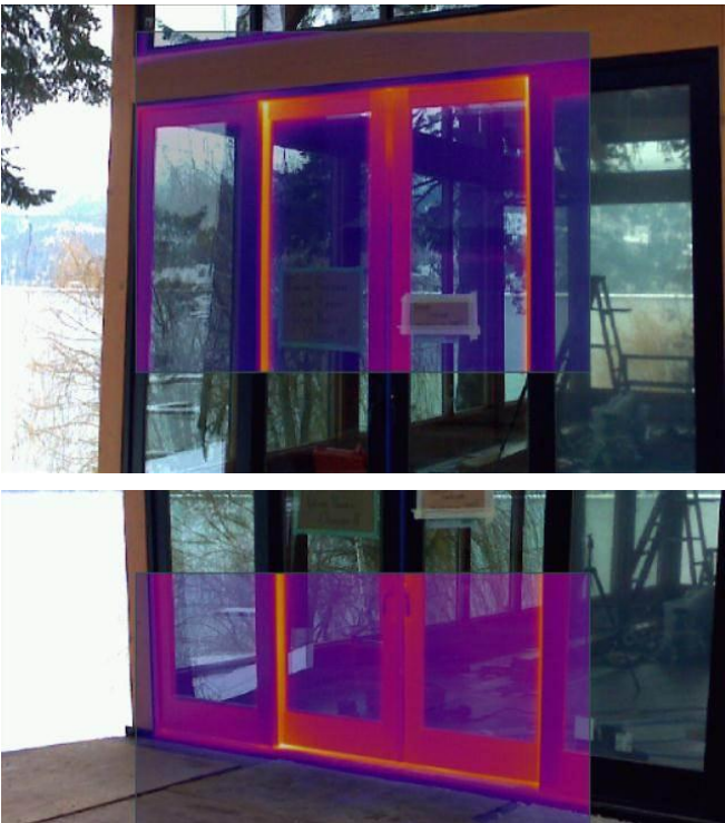
Fig.3.20 IR photo of a sliding glass door during depressurization (left) and pressurization (right), showing air leakage during pressurization around the door frame.
