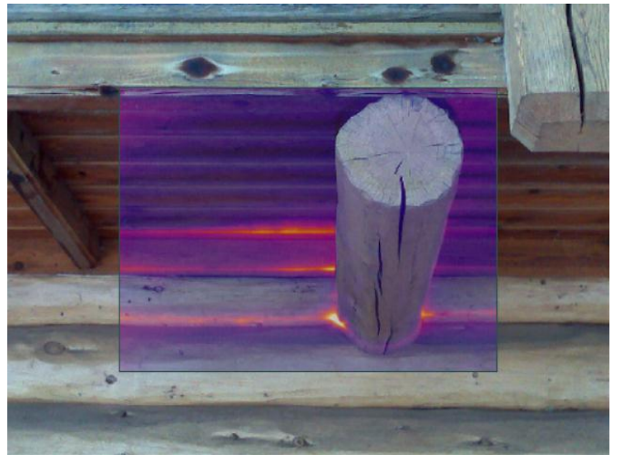
Fig.3.14 Air leakage at second floor door and at roof overhang joints under pressurization.
