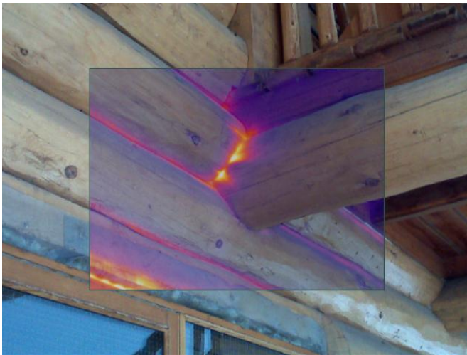
Fig.3.15 Air leakage at joints under pressurization.
