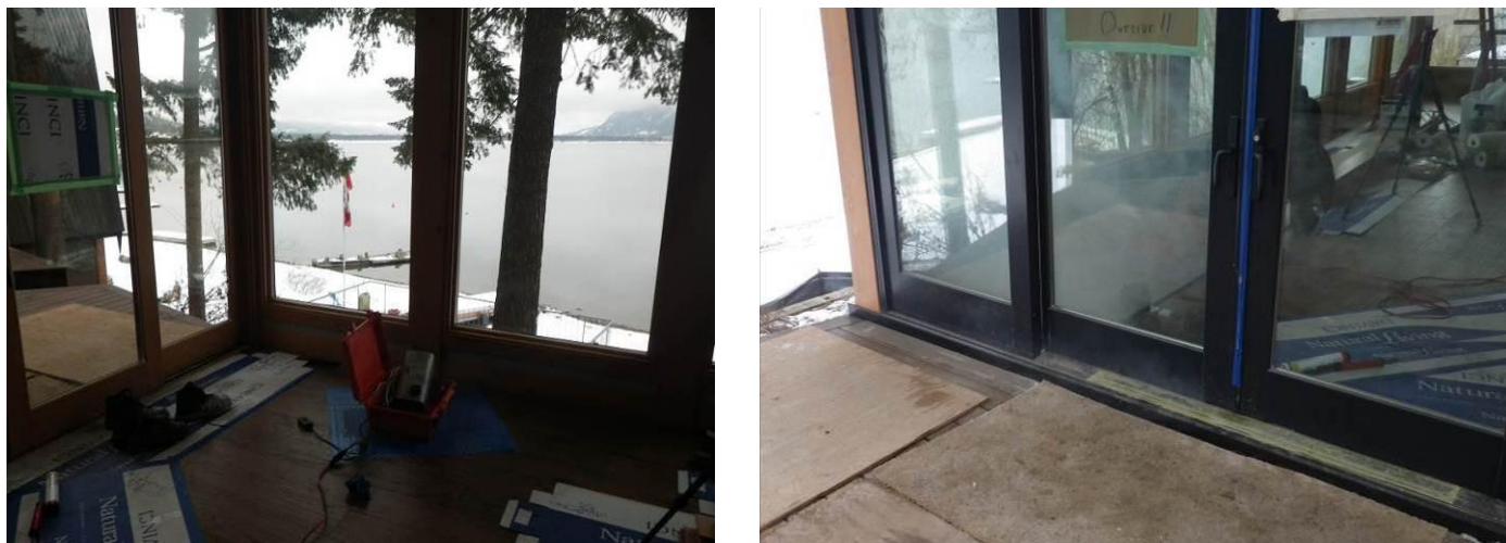
Fig.3.19 Theatrical fog machine used for smoke testing at a corner of the house (left) and smoke leakage observed around the sliding glass door (right) under depressurization.
