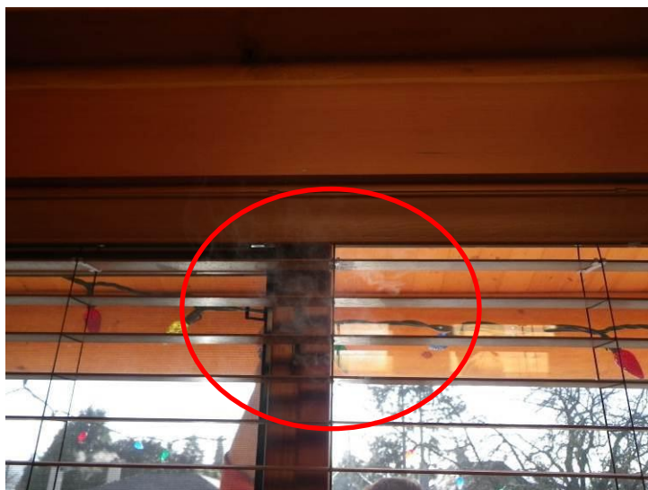
Fig.3.27 Smoke infiltration observed at corner joint during smoke testing from the interior under pressurization.
