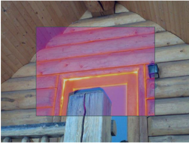
Fig.3.14 Air leakage at second floor door and at roof overhang joints under pressurization.
