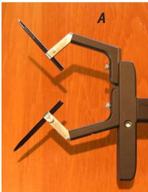
You can position the two Slider arms anywhere along the Female Slide that you want. If you find that the Female Slide gets in the way while scribing a notch (for example), then position BOTH Sliders higher (Photo A) or BOTH Sliders lower (Photo B) on the Female Slide.
