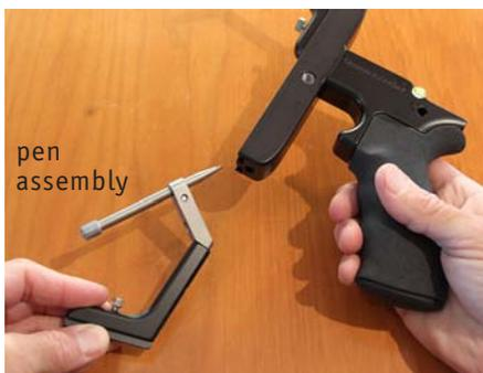
**Step 1 :** Remove **one** Slider from the scriber, and put a pen tube (with refill) into the arm.
