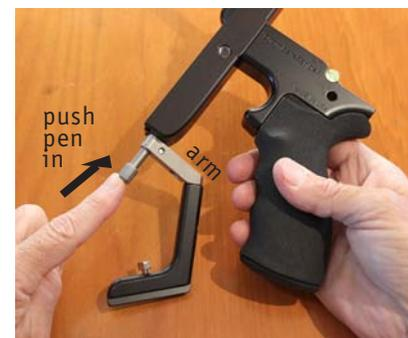
**Step 3 :** Push pen assembly into hole until it stops. Hold the pen arm **tight** against the bottom of the Female Slide. Tighten screw to hold pen tube in place.
