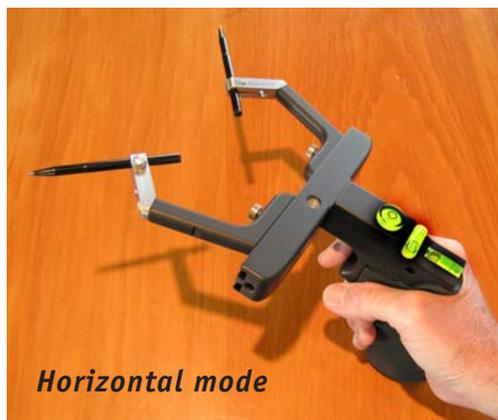
Use either the front straight vial (#2) or the bullseye vial (#3) to keep the pen points horizontal as you scribe. To keep the scriber **pointing** the correct direction you might want to use a laser pointer while horizontal scribing. The ChambersScriber has a hole (#14) that can hold a .25 caliber “bore sight” laser. A bore sight laser is a tool that is used to adjust, “sight in” a telescopic scope on a rifle.
