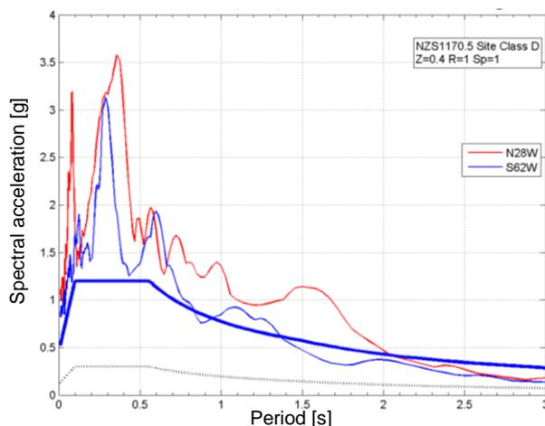
Figure 1: 5% damped elastic acceleration response spectra at the Te Mara Farm Waiiau station (WTMC), horizontal PGA = 112% g, vertical PGA = 322% g. Solid line ULS, dotted line 0.25 ULS for soil class D [1]
