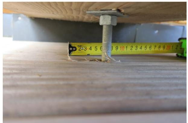
**Figure 23: Sliding of the logs measured at the vertical rod**
